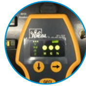
Displays H N G polarity
