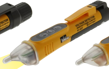
61-637 Single Range 24 to 600V AC NCVT w/Flashlight CAT IV 600V
