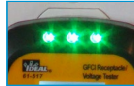
Green Lights Indicate Correct Wiring
