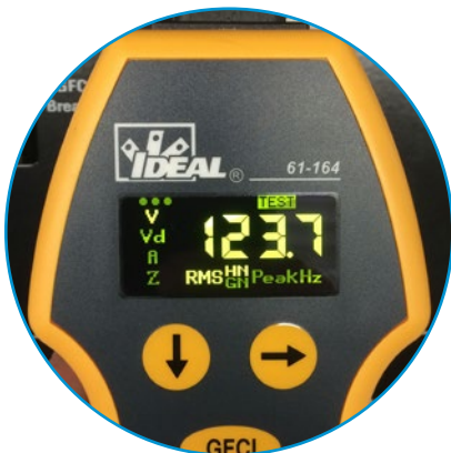
True RMS Line Voltage
