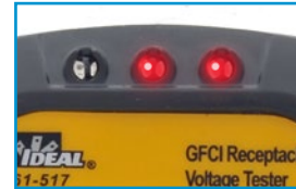
Red Lights Indicate Incorrect Wiring
