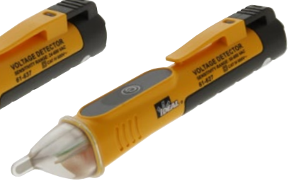
61-627 Single Range 50 to 600V AC NCVT CAT IV 600V
